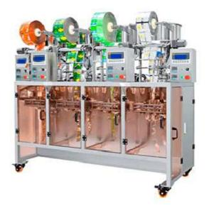
It is suitable for automatic packaging of granules, liquid pastes and powder products in cosmetics, food, health care and pharmaceutical industries. The two machines are packaged in parallel, which is suitable for customers with small sites, large production capacity and little investment in the early stage;
