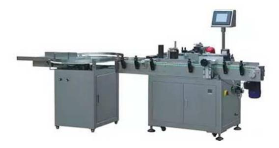
LTB-C is economical, self contained, easy to operate, equipped with touch screen & PLC Control System. Built in microchip storing different job setting makes fast and easy changeover. This automatic labeling system is ideal for small cylindrical container with diameter from 12mm to 45mm such as vials or eye drop bottles.
