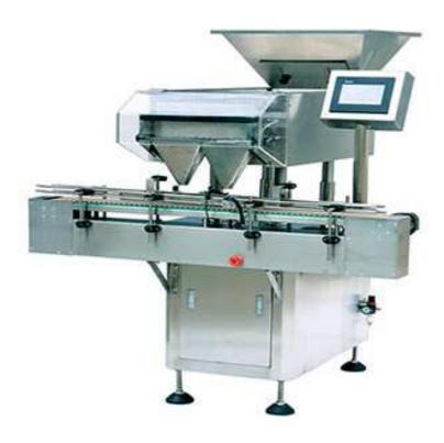
This is one kind of full automatic electric bottle filling and counting machine, which can consist with unscramble, cotton inserter/desiccant inserter, capping machine, induction machine and labeling machines.it can finish the whole full automatic production process.
