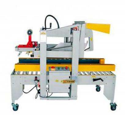
Automatically fold the cover and adjust the width and height after receiving. The carton is suitable for the pipeline operation, the box box is folded and sealed once, without manual participation, the automation is strong, and the two conveyor belts are divided into right and right parts.
