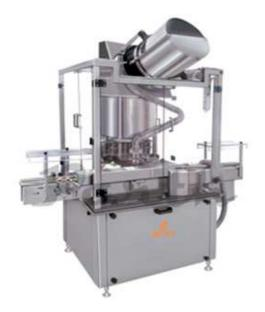
Automatic ROPP Cap Sealing Machine is versatile, self-supported on stainless steel leg with height adjustable adjustment system. The ropp capping machine is precision built on sturdy welded MS frame completely enclose in stainless steel sheet and doors are providing to facilitate the servicing of machine.
