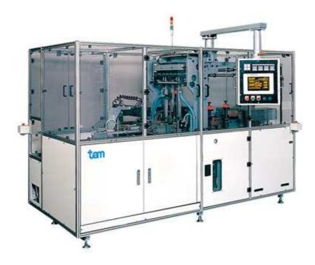
This model has 5 common patterns to be chosen for accumulation (see below) and style can be also selected to lay accumulated items either on edge or lay them out in a flat line. Depending on the products most appropriate pattern will be offered. Automatic feeding device can be equipped as pre-process to collect and accumulate single or double layers to transfer to the W4202 overwrapping machine.
