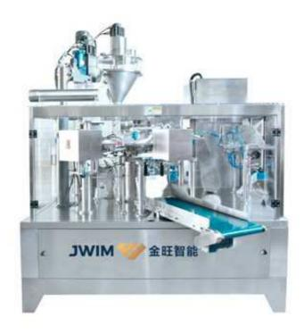
The machine is making up with the automatic packing machine and filling system. It has wide application range and can pack liquid, powder, granule and solid products by changing different dosing system. The machine can change different packing volume in short period of time. The auto pouch feeding width can be adjusted by the handle. The machine is with inspecting device to make sure no fill and seal if the pouch is not opened successfully. This will save the pouch and products.
