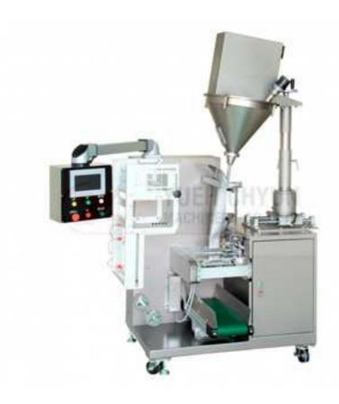
The machine is servo continuous motion with three axis servo motor system to easily setting up and programmable logical controller to allow additional facilities add-ons when needed. With the auger dosing system, it is suitable for powders. The packing machine could also be equipped with different dosing system according to the product conditions.
