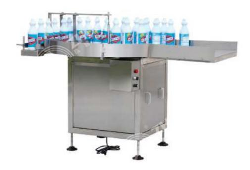
This rotating bottle feeder machine is use eccentricity from disc rotation, it will send the bottles to the conveyor under the action of bottle guide board, then into the next process. This machine is suits for  $\Phi 30$ -100mm cylindrical shape bottle unscrambler. Machine use frequency to adjust speed, the whole machine use SS304 and with long durability. Unscrambler speed can achieve 7000 bottles/hour.
