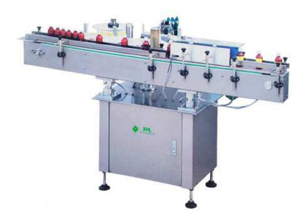
This series machine is applied to glass & plastic round bottles. In the field of pharmaceutical, pesticide, chemical, foodstuff etc. It is able to auto separating bottle, feeding label belt, separating label, sticking and auto printing codes. It is equipped with large torque step in motor of servo motor and imported photoelectric controlled PLC to ensure the accuracy, stability, reliability, and high efficiency.
