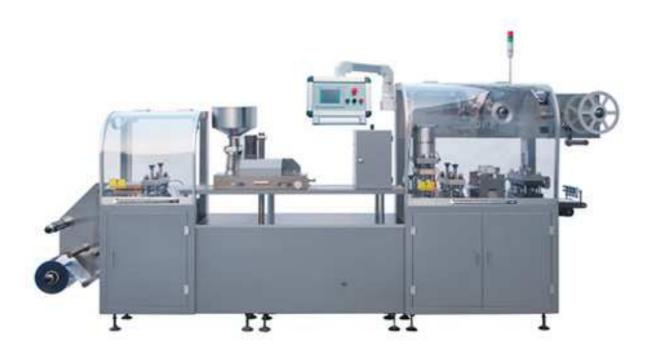
The design structure of DPP-260 series automatic blister packing machine is meeting the standard requirements of GMP, cGMP and the design principle of ergonomics. It adopts advanced smart driver and control technology.
