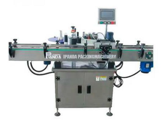
Automatic bottle labeling machine for can bottles is applicable to chemical paint pesticide cylinder, bottled water, cooking oil and other cylindrical objects. Rubber wheel divide bottle, equidistant spacing, labeling is more accurate. Wheel attached to the roll on bottles, make label attached more firmly.
