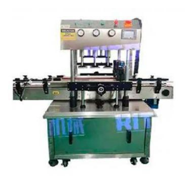
High speed capping machine is a new type of capping machine, with reference to the international advanced model to improve the design, fast capping speed, high pass rate, easy to operate, high technology content, stable performance, reliable quality. Four speed control motors are used for capping, bottle clamping, transmission, capping, machine automation is high, stability is good, easy to adjust, no spare parts are required when changing the bottle shape or cap.
