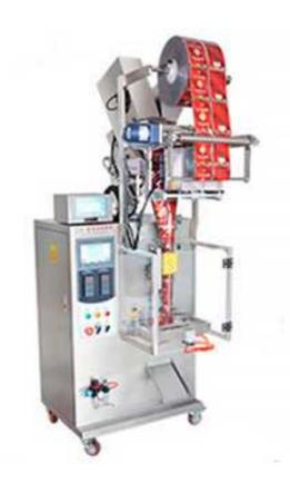
The packaging machine is an automated equipment that automatically completes bag drawing, bag making, filling, metering, sealing, bag cutting, counting and coding during the packaging process.
