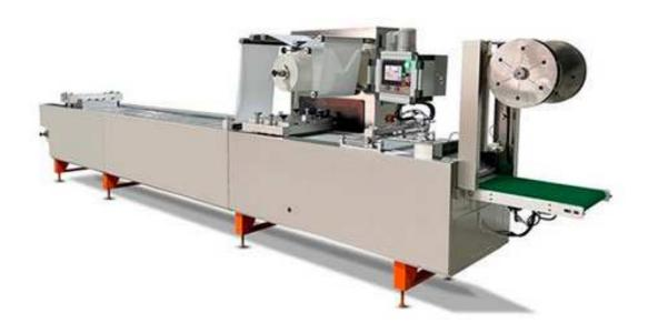
GTI-P420 Blister Packing Machine adopts PLC processor, temperature module, servo main motor, and big color touch screen control.
