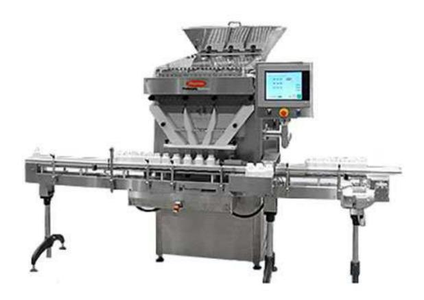
The Pharma Packaging Systems Model SuperCount 18-3 is the latest evolution in electronic tablet counting, combining proven technology with the latest in electronic control systems including 'onboard' microprocessor for the highest level of reliability.
