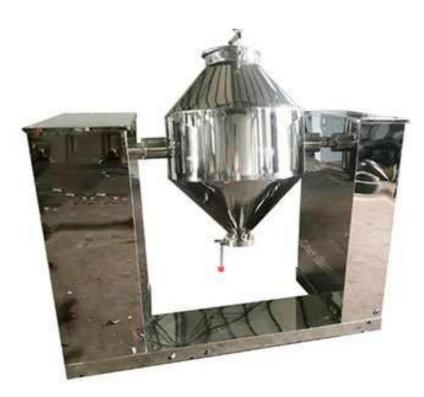
The mixing barrel of W type Mixer Machine is designed to be double cone shape. When the barrel rotates, the dry powder or particles are continuously lifted in the barrel, and then thrown and staggered to achieve rapid and uniform mixing. The material to be mixed by the double cone Mixing Machine must be dry material with fluidity. If you want to mix agglomerated materials or materials containing a certain amount of liquid, you can choose WI series Industrial Blender.
