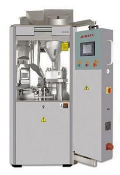
This series of Capsule fillling Machines adopts a programmable control system, touch screen panel, speed-shift and electronic automatic counter.
