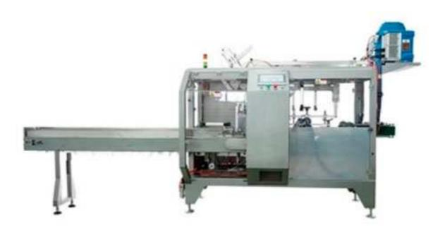
HTZH-200 Automatic Boxing Packing Machine is automatic high speed continuous cartoning machine which is high performance product incorporates pneumatic, photo, electric, and mechanic in one.
