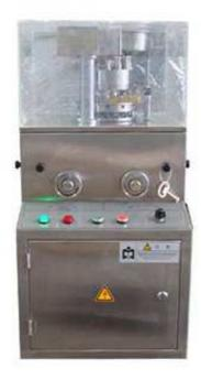
Meeting the GMP standard, ZP type tablet presses are ideally-designed to press granular raw materials into round, non round tablets for laboratory use for laboratory use for research and development or small-scale production in pharmaceutical, chemical and food industry.
