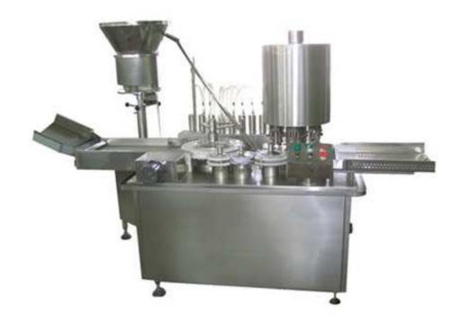
This machine is the main filling & sealing equipment of the oral liquor production line, which is mainly applied in the filling and sealing of 10 ml or 20 ml bottles.
