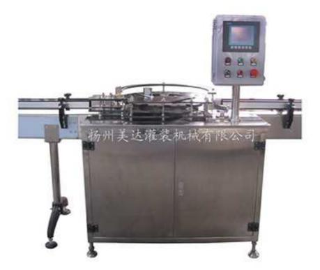
The machine can weigh each can of aerosol, and isolate those cans in which aerosol weight is not with in allowance.
