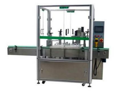
This Perfume Automatic Filling Machine is specially designed for the filling of perfume vials. It uses a peristaltic pump for liquid filling, plugging and capping. The machine can be used in pharmaceutical, medical and cosmetic production plants. The machine can automatically complete the bottle unwinding, bottle transportation, filling and stopper feeding, plugging, bottle cap feeding and curling.
