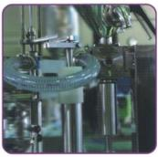
The filling amount can be adjusted even during operation and easy to disassemble for cleaning
