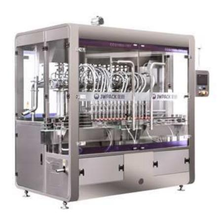
CCG1000-16TS Automatic piston filling machine is the upgrade volumetric filling that can be widely used for the high viscosity filling of liquid, it is used for the chemcial product filling from 80ml-1L, the servo motor driven and Schneider Control System can make the stable and high precision filling. An optional functioned high precision electric scale weight feedback system makes the volume adjusting easier and more convenient.
