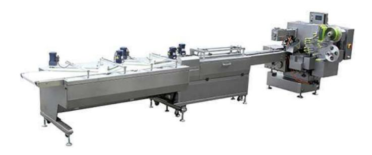
FW-820C uses feeding conveyor and feeding plate, solves the problem of those chocolates and candies which are hard to be fed by vibrating wheel bowl.
