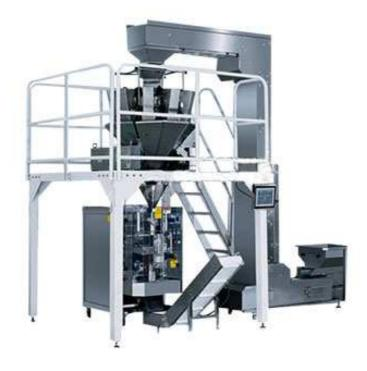
Automatic food packing equipment is specially designed food packing equipment based on advanced technology. It is a perfect combination of vertical packaging machine and ten heads combination weather, which can realize whole process automatically from weighing and filling to bag making and packaging. Our automatic weighing and packaging unit plays significant role in food processing industry and is your reliable choice.
