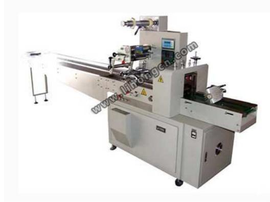
Flow Pack Machine – GZB model design provides for packaging of piece products in 3- side bags. This machine is suitable for individual product as well as group product in container (tray). Bags are made of heat seal film in rolls.
