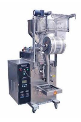
The machine is designed and manufactured specially for water, honey, oil, sauce, jam or similar liquid products. Driven by servomotor, the piston back and forth to fill liquid; furthermore, the filling range can be adjusted automatically through computer The processes of bag making, measuring, filling, sealing, cutting, counting and hot pressing codes can be done automatically. Packing material include several kinds of heat-seal lamination, such as PET/plated AL/PE, PET/PE, NYLON etc.
