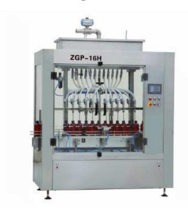
Accurate measurement: adopt servo control system; ensure the piston can always reaches constant position
