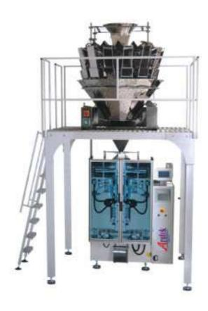
With this machine you can pack your granule or vulnerable products (sugar, salt, pepper, instant coffee cream) by weighed system fully automatically. With this machine you can make quarto, pillow and standup pouch packs.
