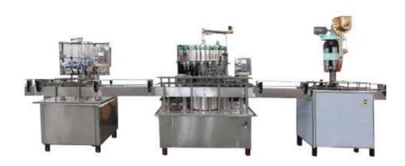
This Liner type filling machine is specially designed for Water /Juice / carbonated beverage, Filling type is Normal pressure or Count pressure. All parts of this machine is made of stainless steel materials, it cannot cause rust to influence the filling beverage, it not only reach the standard of sanitation, but also prolong its using life.
