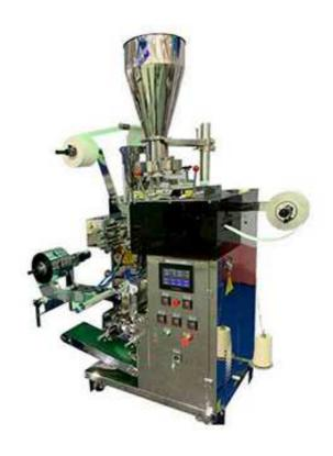
This tea bag filling sealing machine is suitable for the dual bag packing of small grain-like materials, such as tea leafs, medicinal tea and healthy teas. it can finish bag making, tea leaf filling, tea bag inner sealing with tag, tea bag filling, 3/4 side outer seal, coding in one machine.
