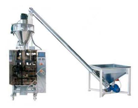
This powder filling packing machine is suitable for packing powder products, such as wheat flour packaging, milk powder packing, detergent washing powder packaging, fruit powder packing etc.
