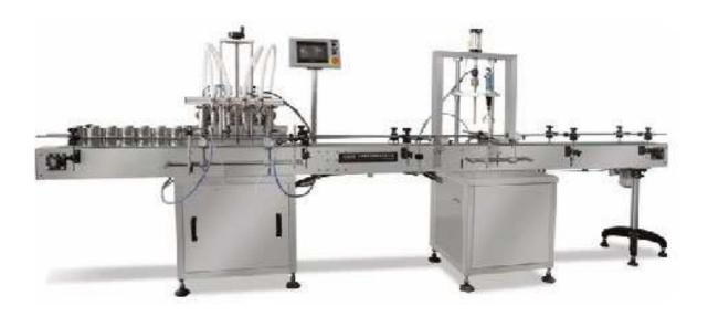
Semi-Automatic Capping Machine is designed for the PET screwed caps, the size of the capping heads are based on the size of the caps.
