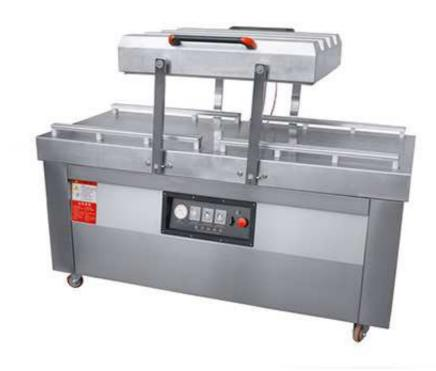
DZ-700/2SA double chambers vacuum packer can finish the whole programs of vacuum extraction, gas injection (optional), sealing, cooling and exhaust automatically. The products after packing can be prevented from oxidation, going mould, insects or getting damp, thus can be kept fresh for longer time. This is an efficient, sustainable double chambers model for outstanding vacuum packaging results.
