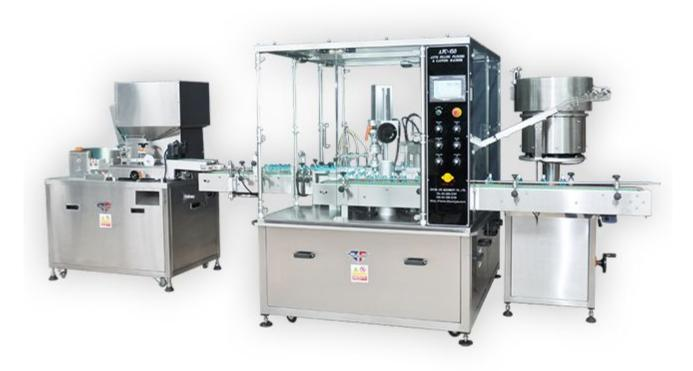
The liquid production processors design compliances with cGMP of the liquid product guideline. The processors are applicable for low viscosity and volume below 60mL.
