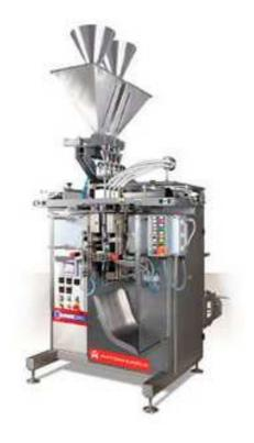
PLC control unit, servo motor controlled film transport, connection apparatus and hoses for aspirator group. Metallic grey colored and surfaces of the machine that are in contact with the product made stainless
