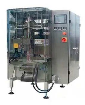
VFFS-240 Automatic Vertical Form Fill Seal Packaging Machine is widely used for small-particle material packing, can make various of bags, the max bag width is 180mm, the maximum speed can reach 90bags/min.
