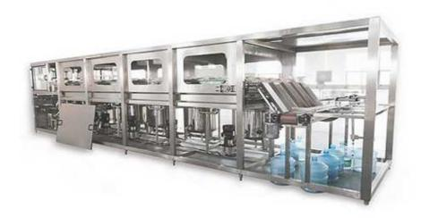
This automatic mineral water filling machine mainly used in the water filling operations, the three function of bottle washing, filling and capping are composed in one body of the machine, the whole process is automatic, it is conveniently trunked to adjust the machine to fill various types of bottles, the filling operation is faster and more stable due to the advanced filling valve technology, The famous brand programed controller (PLC) is adopted to control the machine runs automatically.
