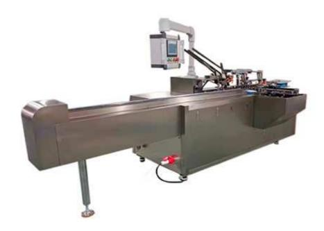
PZH-120H Automatic cartoning machine is a high-performance product that integrates electromechanical, gas, and light-based on foreign advanced equipment introduction. It meets GMP requirements. The machine is a continuous operation, automatic box opening, leaflets automatic folding(1-4 folds), printing batch number sealing detection and other functions (can also be equipped with hot melt adhesive device), the highest speed up to 90-110 boxes/min.
