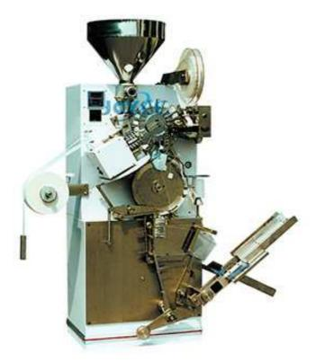
This is our high speed automatic tea bag packing machine, it makes filter tea bag with cotton thread and tag, the speed 120bags/min, with auto boxing device included, there is vacuum feeding device, heat sealing tag device, stirrer, date printing machine optional.
