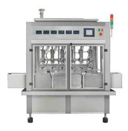
CZ-6 full Automatic Weighing type filling machine is suitable for liquid barrel packaging. Each filling unit has high-precision weighing sensors, control instruments and filling speed control valve, which can adjust the filling speed as required.
