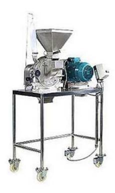
PMS PIN MILL® is used for fine to very fine grinding of dry, brittle and non-abrasive materials. The size and throughput of the ground material is controlled by pin and disc configuration, sieve and rotor speed.
