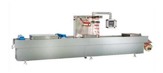
Thermoforming vacuum food packaging machine is suitable for fully automatic continuous packaging of food packaging. Whether it is soy products, bulk meat in slaughter and cutting operations or continuous vacuum packaging of dairy products.
