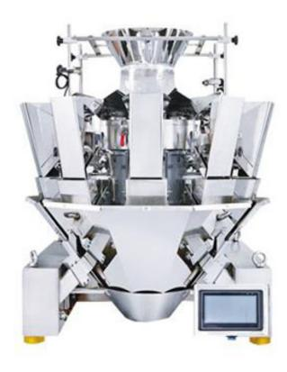
The 10 head multihead weigher has a weighing range of 10-1200g and a maximum packaging speed of 65bags/min when used together with the vertical bagger. This weigher is perfect for a variety of granular, sheet, strip and irregular products such as confectionary, potato chips, jelly and more.
