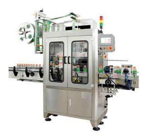
Cap Tamper & Body Shrink Sleeve Labeler is designed for bottle cap sleeves & full body sleeve. It can be used in various bottle sleeves and different sleeve positions. The production speed of PTB-250p sleeving applicator is 0-15000bph.
