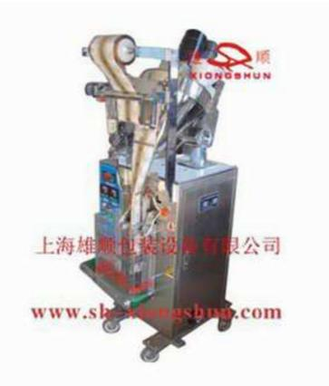
Step motor controls filling-screw to reach high precision. The whole measure system is controlled by step motor too. This series machines are used to packing powder. Products such as pesticide, fertilizer, medicine, facial mask, dried milk, spice and so on. Screw filling is suitable for bad fluidity material and owns feature of high speed, accuracy and practical use.
