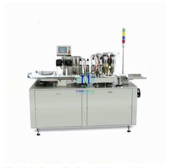
The E-Liquid Filling Machine/Eyedrops Filling Capping Machine is suitable for plastic and glass bottles of various shapes. PLC controlled peristaltic pump filling. It functions as the new generation equipment of eyedrops production in the pharmaceutical industry, but is also used for packing small dosage liquid for other industries.
