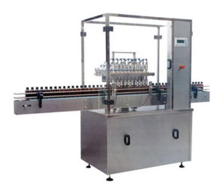
This machine is suitable to wash the circular or quite regular plat ode plastic bottle. It can clean out the dust and plastic granule in the bottle. This machine adopts touch screen interface and photoelectric control. The air which is used to clean the bottle circles in and it will not pollute the workshop's environment. We can equip with vacuum pump and dust shield according to the client's requirement. It can be changed into a big volume liquid filling machine.
